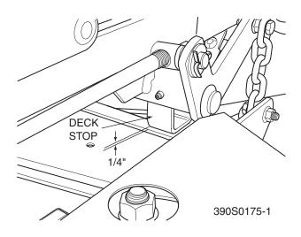
Figure 6-8. Cutter Deck Stop
